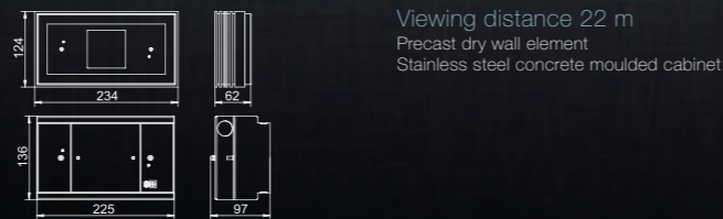
Viewing distance 32 m Precast dry wall element Stainless steel concrete moulded cabinet
